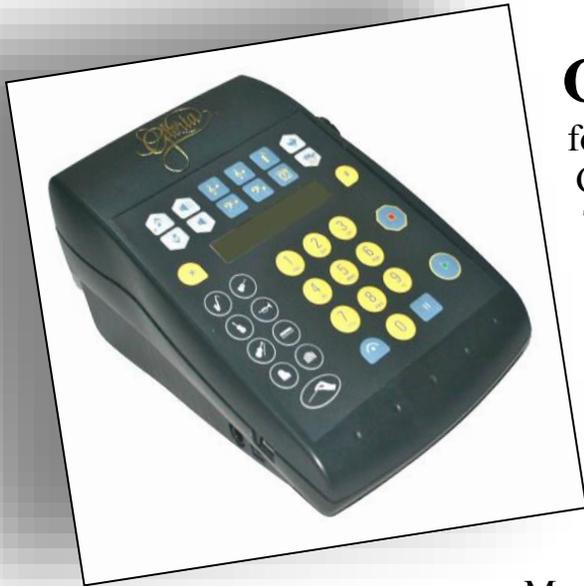
**GLORIA3** is totally self-contained. It runs on four D size flashlight batteries or an AC adapter. Gloria has a built-in speaker with a 5-watt amplifier. The volume from the speaker is adequate for a group of ten to twenty people. For use in larger churches, a sound system, keyboard amplifier, or guitar amplifier can be plugged into the external audio jack.
